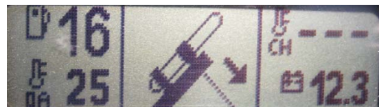
powerplant in position propeller stopper extended
